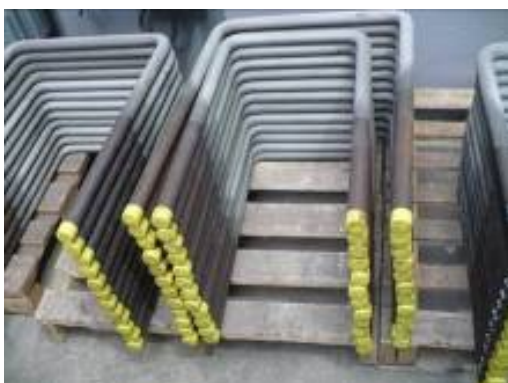
Fig. 12 Arc sprayed boiler tubes (left) and Castolin Eutectic arc spray booth (right)
