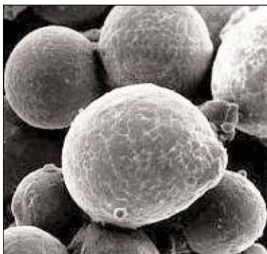
Photomicrograph shows a dense coating with a high volume percent of uniformly distributed, discrete tungsten carbide particles.
