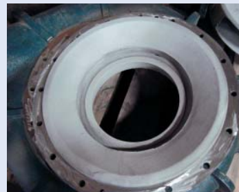
Coated pump housing to resist erosive wear and cavitation.
