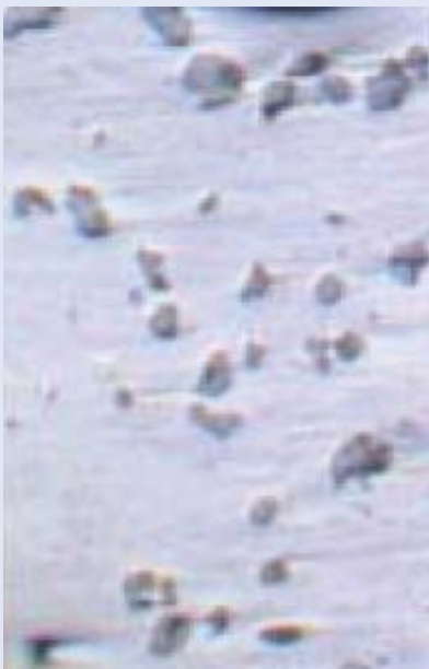
Undiluted Tungsten Carbide particles after welding (33 HRC matrix).
