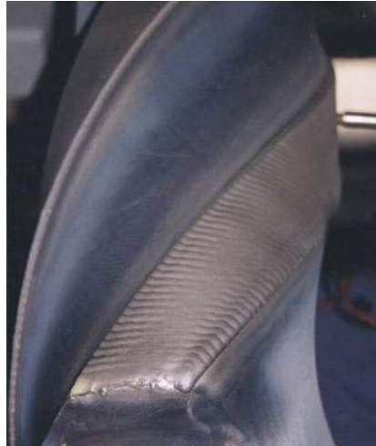
Stabilizer Protected with SF Lance
