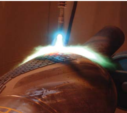
Stabilizer with Carbides being Sprayed
