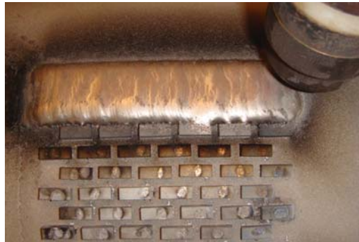
Tungsten Carbide Tile and PTA Weld Flood
