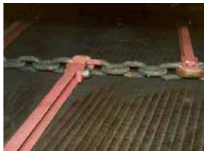
Chain conveyor bed
