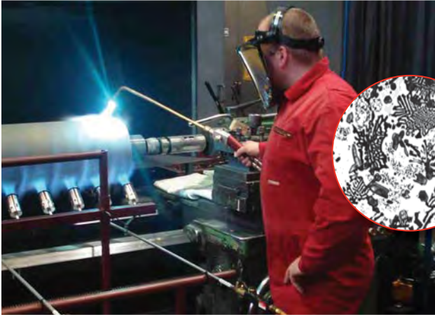
Spray and Fuse Process (TeroDyn® and SuperJet®)
