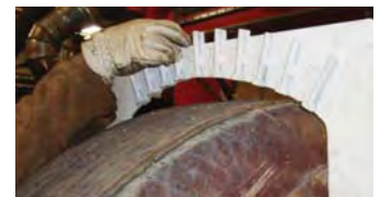
Material loss caused by abrasion
