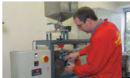
Lab testing to define wear resistance
