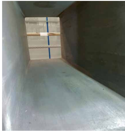
XuperCOAT™ applied on a bloom mould; coating condition after 600 heats
