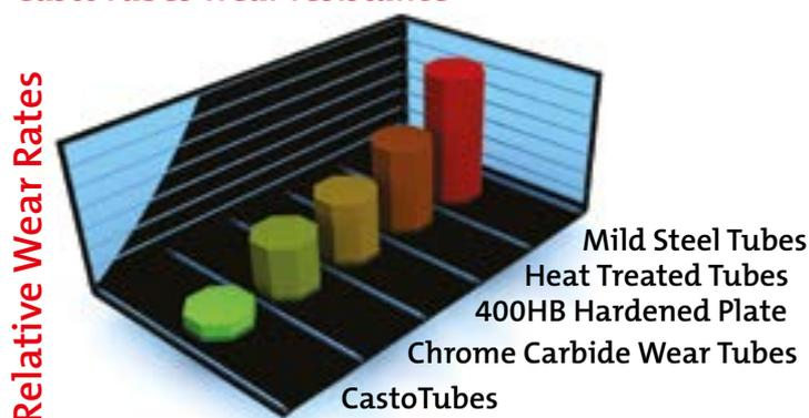
CastoTubes are engineered for exceptional wear resistance as illustrated by the laboratory abrasion wear test data above. This performance results from:
