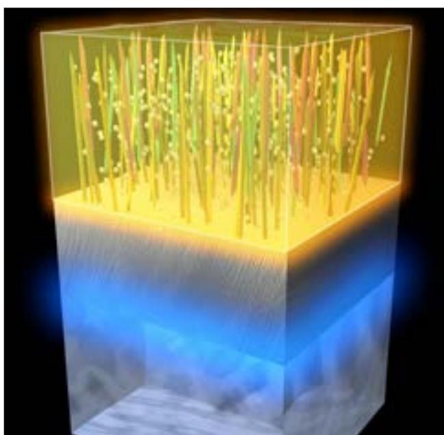
Controlled cooling during the manufacturing process produces densely dispersed hard phases. These are strongly oriented to provide superior wear resistance to conventional weld coatings.
