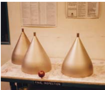
Power industry: Parts protected with vacuum fusing
