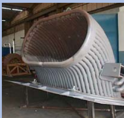
Furnace duct for the steel industry protected against heat and erosion
