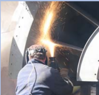
Protecting a ventilator against erosive wear
