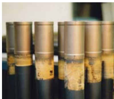
Oil&Gas industry: Parts protected with vacuum fusing
