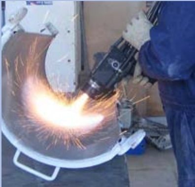
Parts in babbitt being sprayed
