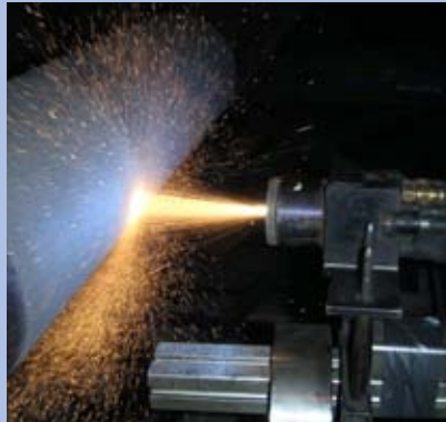
Huge roller being sprayed, efficient solution to protect large areas
