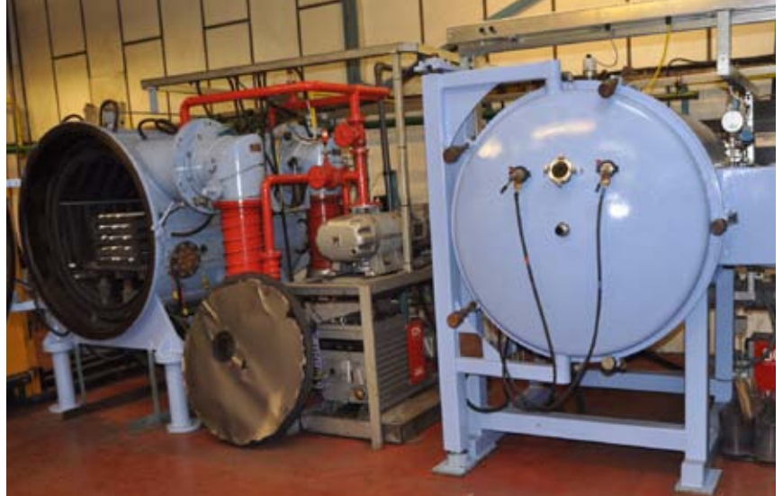
Workshop equipped with 2 vacuum furnaces
