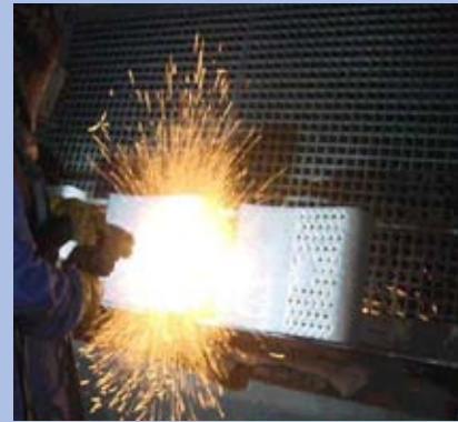
Fuller plate for the cement industry protected against abrasion
