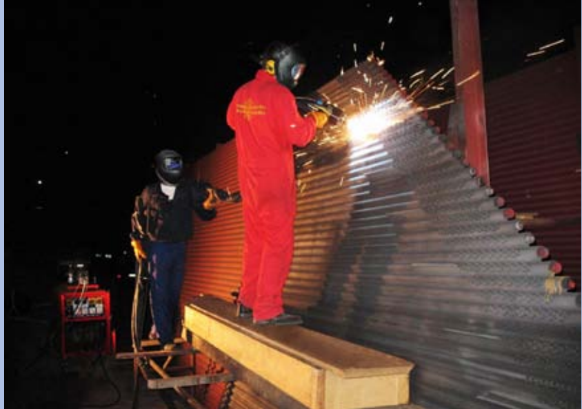
Protected boiler tubes against hot gas erosion and corrosion in thermal power industries
