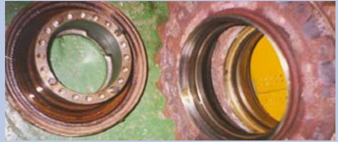
Drive sprocket protected against friction combined with pressure
