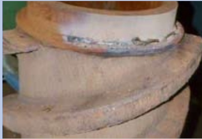
Extrusion screw protected against abrasion combined with pressure
