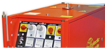
Switched Input Voltage (SIV) fitted in the top compartment
