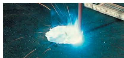
Hole cutting with CutTrode
