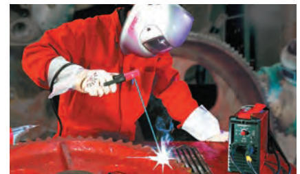
Rebuilding gear teeth
