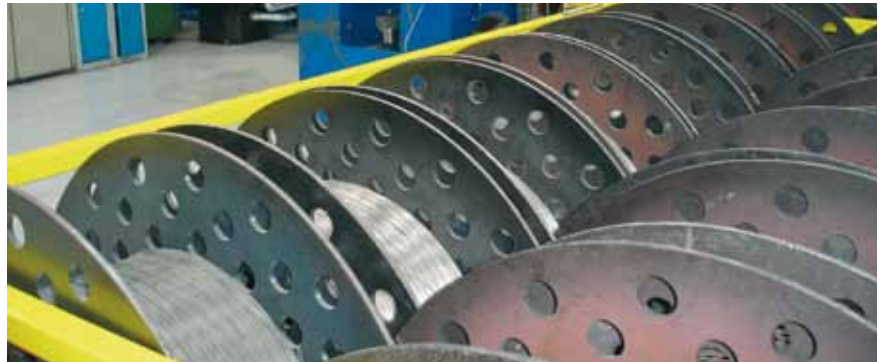
Quality wire awaiting baking to improve surface properties
