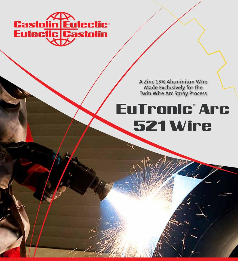
A corrosion protection coating superior to Zinc and Aluminium coatings especially in atmospheric environments
