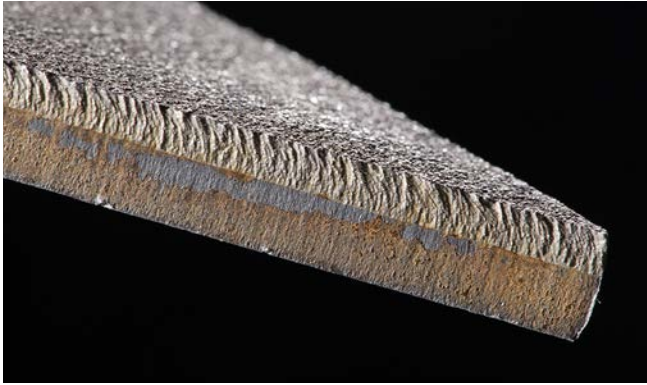
Powder coated CDP®. Visible lack of dilution.
