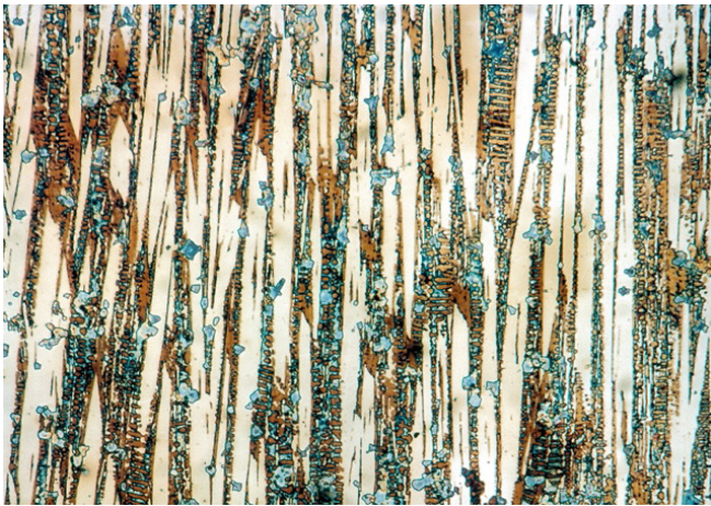
Microstructure of wearplate with densely packed, regular hard phases in tough matrix for better wear resistance.
