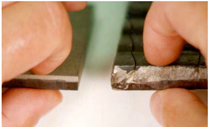
CDP powder wearplates (left side) Are extremely thin and far lighter than a welded wearplate (right side).
