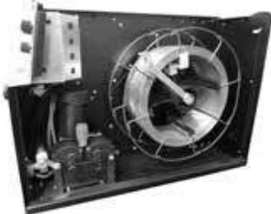
A black and white photograph showing the internal mechanism of the spool carrier spindle brake. A circular component with a central spindle is visible, and a screw is being used to adjust its tension. The mechanism is housed within a dark metal casing. |
