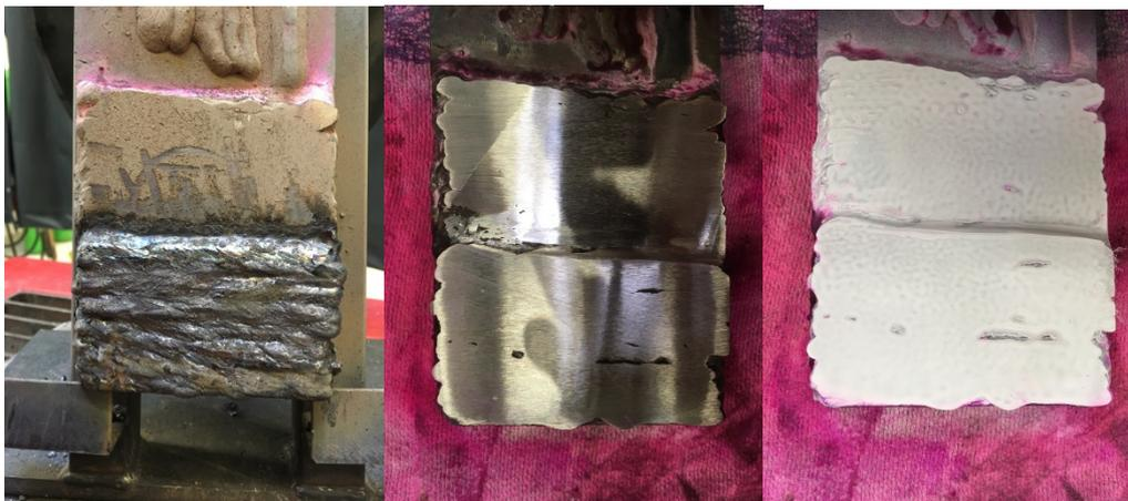
*So welding with old transformator power source with AC current or with CastoTig with MMA AC setting is giving good result without porosity for Cavitec SMA instead DC (+).*
