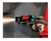
The ArcJet fits on the gun to inject air in front of the nozzle. The ArcJet constricts the spray pattern thus reducing overspray and allowing more confi ned areas such as deep slots, to be sprayed.
