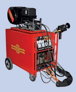
EuTronic Arc is the highest productivity thermal spraying process. EuTronic Arc is an Arc Spray Process using a pair of wires which are melted by an electric arc.
