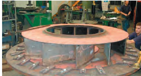
Fan built with wear resistant CDP
