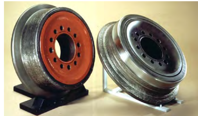
Frictional wear of wagon wheel flanges in railways
