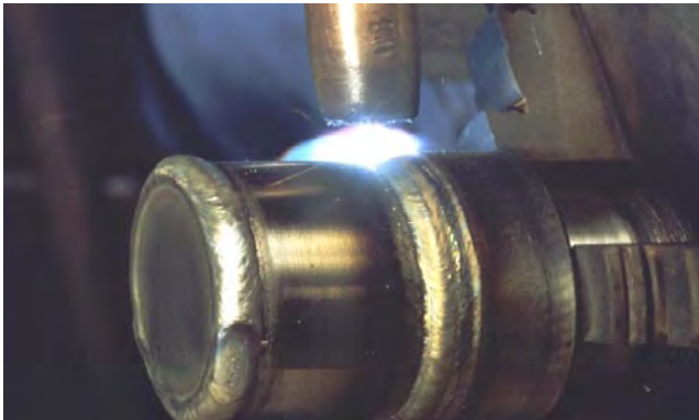
Wearfacing a plunger component
