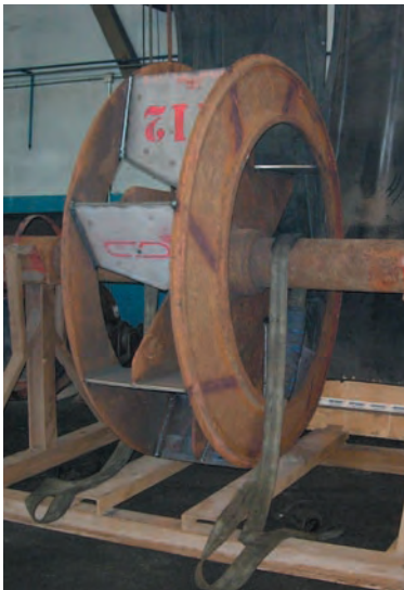
Fan Protected with Powder Coated Wear Plates
