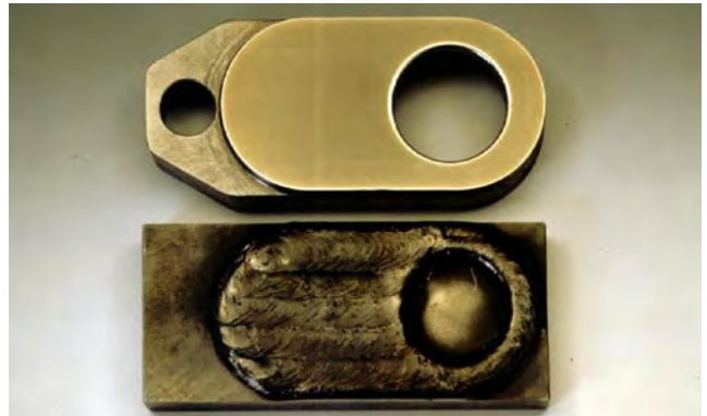
Petrochemical OEM weld protected gate valve for corrosion resistance
