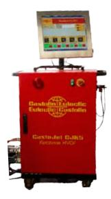
The CastoJet® Kerosene 5 - CJK5 - is the latest Castolin Eutectic development of kerosene fuelled high pressure HVOF (High-Velocity Oxy-Fuel) systems. Using mass flow control for repeatable coating quality. The system produces the densest metallic and carbide coatings of all. The coatings can be compressively stressed, allowing thick layers to be applied without fear of spalling.
