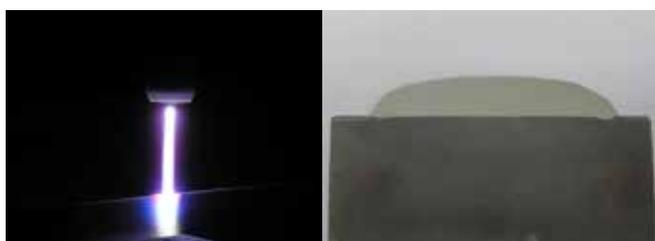
Focused plasma arc allows extra control, that results also in low dilution, smooth surface coatings and spatter-free welding beads: rework and welding material costs are minimised.
