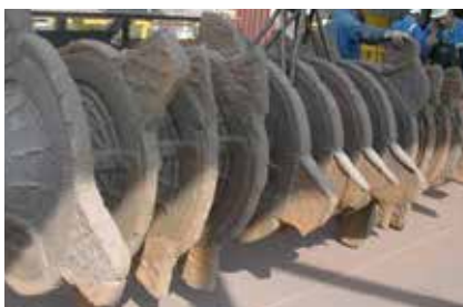
Standard solution after 10 months Rotor is completely worn-out
