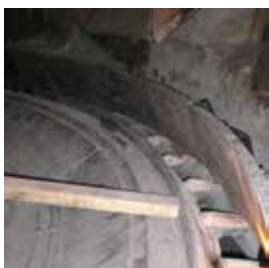
Air guide cone clad with NanoAlloy
