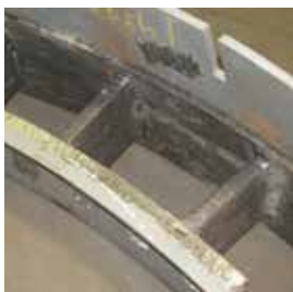
Nozzle ring segment with NanoAlloy protection
