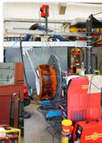
Coating with PTA welding
