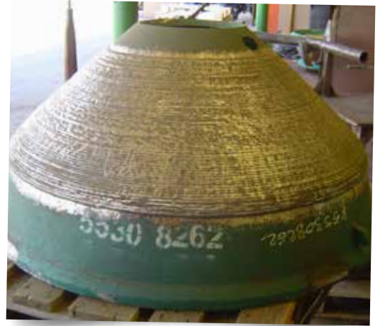
Preventive wear protection of cone crusher
