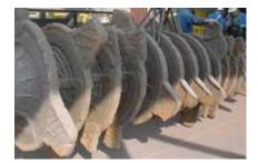
Standard solution after 10 months Rotor is completely worn-out
