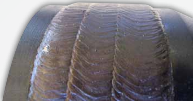
OTW 10SS hardbanding alloy applied on a tool-joint
