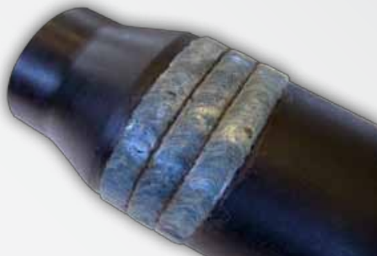
OTW 12Ti hardbanding alloy applied on a tool-joint
