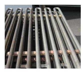
The FuseClad coated tubes do not need any boiler tube shells (usually installed to protect against soot blower wear) which leads to an increase of the heat transfer.
