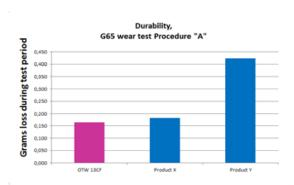
Product X\* - Replacement to an earlier cracking type alloy Product Y - designed to be crack free
