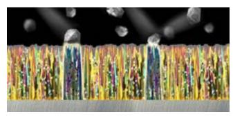
Dense dispersion of strongly oriented hard phases maximise wear resistance
